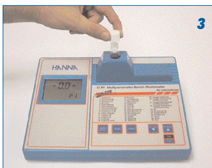
Place the vial in the HANNA instruments® photometer and read the result on the LCD
